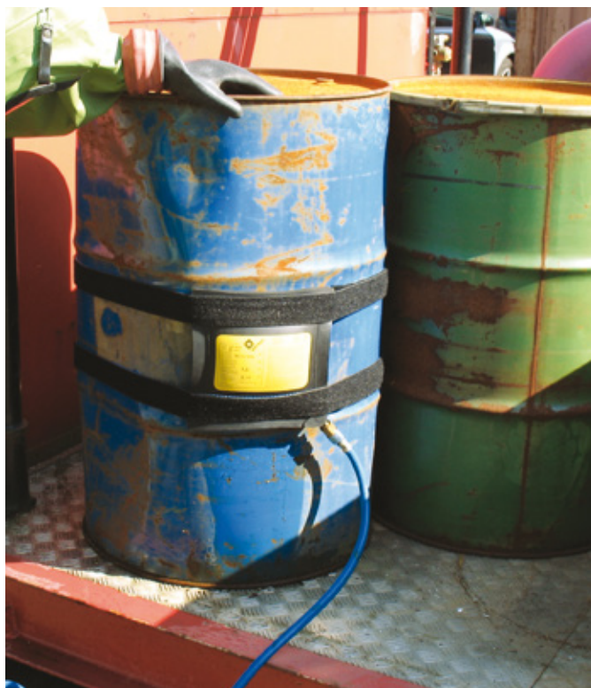
Sealing bags stop leaks in drums
